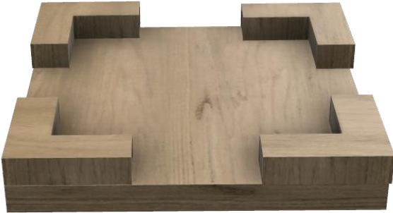
(a) Lower platform with Option 1 L-shape wooden supports for increasing height.
